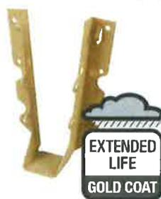
**Gold Coat** is a proprietary multi-layer protection system. It is comprised of an organic top coat barrier layer and a zinc layer placed over a steel substrate. Use with Gold Coat or Hot-dip galvanized fasteners.
