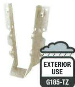
**TZ galvanizing** provides a prefabrication coating of 1.85 (G-185) ounces of zinc per square foot of surface area (both sides) measured in accordance with ASTM A 653. Use with Hot-dip galvanized fasteners.
