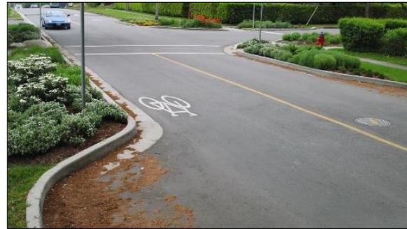
**FIGURE 5M: CURB EXTENSIONS OR BUMP OUTS AT INTERSECTIONS REDUCE THE CROSSING DISTANCE FOR PEDESTRIANS AND SLOW TRAFFIC, INCREASING CROSSING SAFETY, ESPECIALLY FOR THOSE WITH PHYSICAL LIMITATIONS.**
