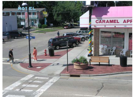
Figure 2. Curb Extension at a Street Intersection
